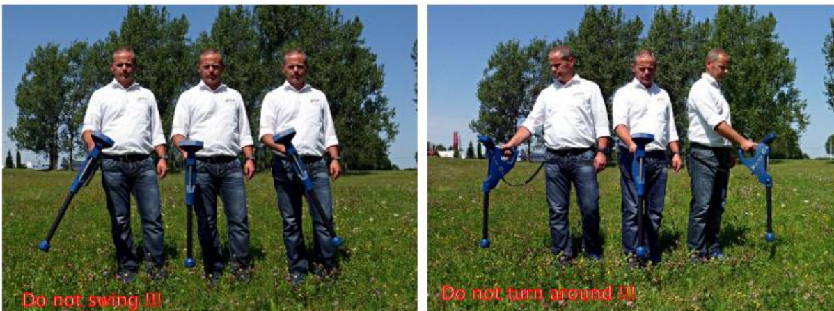
Figure 7.10: Pivoting or turning of the probe falsifies the measurement
